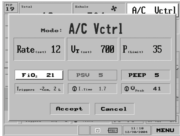
Figure 4.22 \text{FiO}_2 shown selected on the Mode screen (A/C Vctrl) will bring up the \text{FiO}_2 pop-up.
