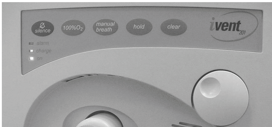
Figure 3.1 The iVent 201 front panel
